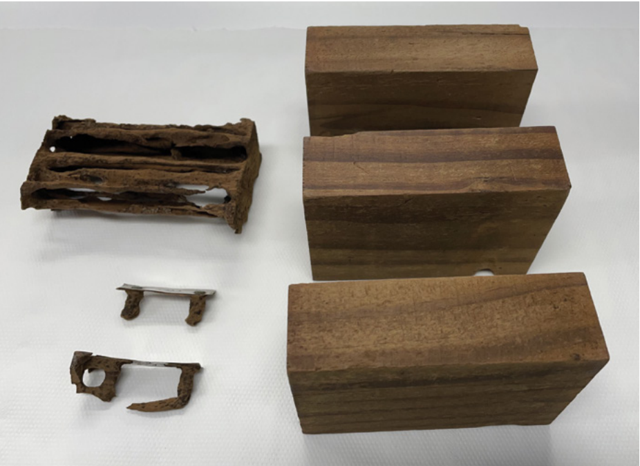
Comparative performance of Imbue Radiata 230 °C untreated (left) vs LOSP Azole and permethrin treated (right), when exposed to Coptotermes acinaciformis termites in AWPC H3 field test, Queensland.
