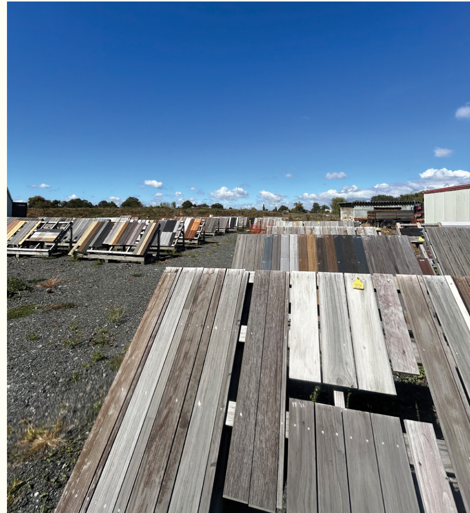
Accelerated weathering exposure, New Zealand.
