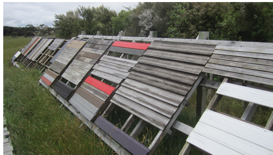
Flat panel test racks, Mangere.
