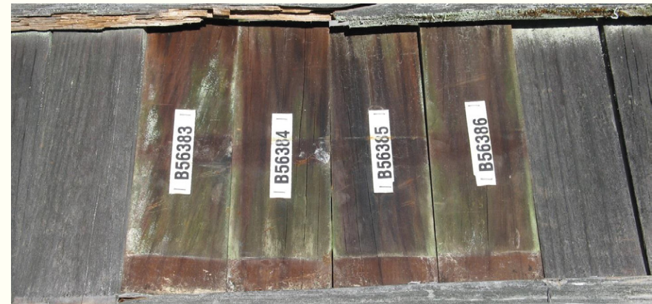
Flat panels Imbue Radiata 230°C after 11 years exposure, Rotorua.
