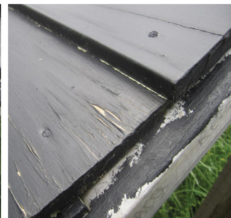
Pressure Treated Clear Grade Radiata Pine, Painted black, 3 years exposure.
